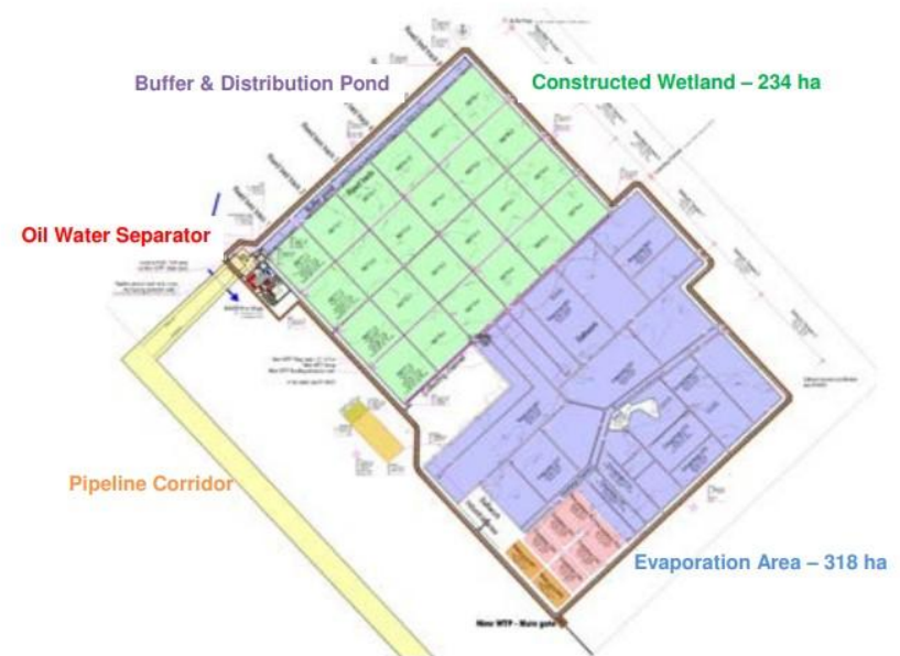
Figure 1: Nimr Water Treatment Plant Design
